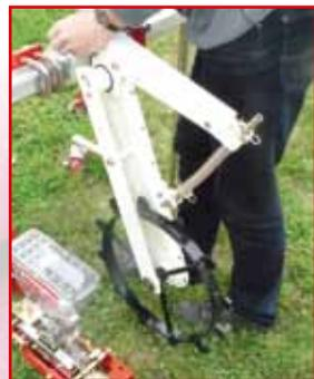
**4** Install the fertilizer driving wheel on the bar.
