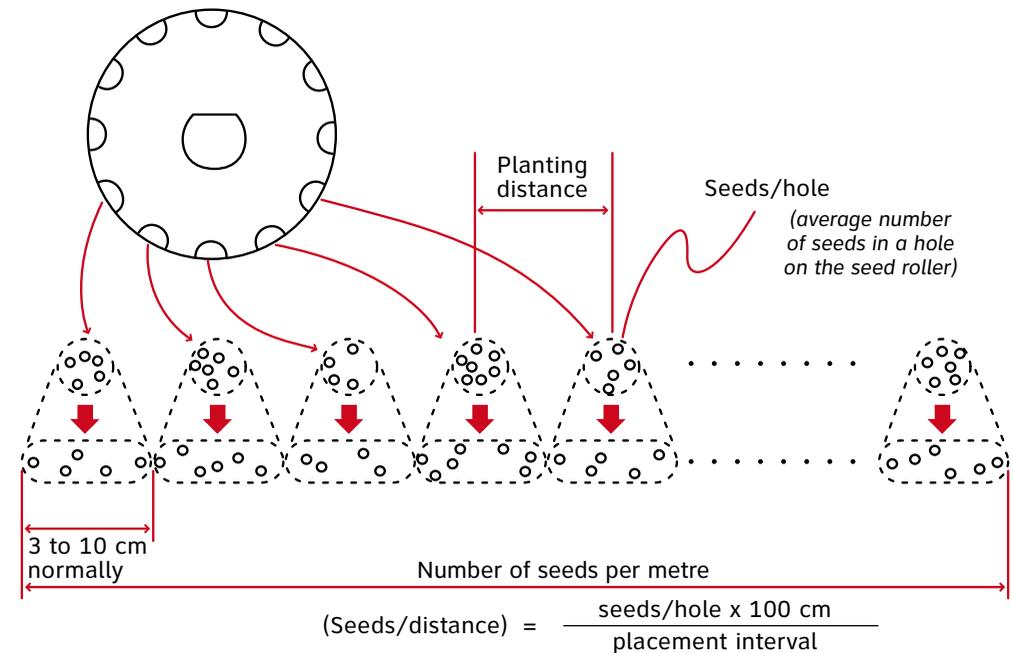
**Caution:** the planting distance depends on the combination of sprocket teeth (11 adjustment positions) and the number of holes on the metering roll. The drive wheel may slip depending on soil quality and placement speed. Therefore, the number of seeds is a guideline only. If the transmission wheel skids, planting distances will be larger, reducing the number of seedlings. So make sure that the wheel does not slip.
