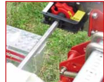
**6** Choose the end fitting the most adapted to your needs and install it at the bottom of the fertilizer hopper in the slide rail.
