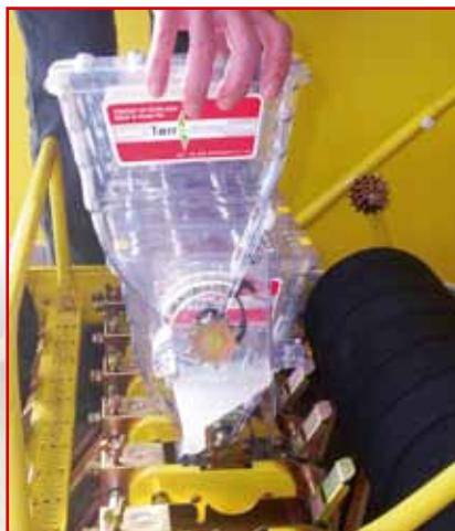
**3** Unscrew the white knob and open the retractable portion of the hopper
