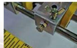
The sowing depth can be adjusted individually for each row by loosening the nuts on the front of the seeding unit.
